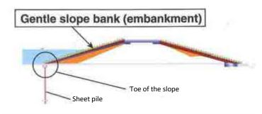
A gentle slope bank is build up by widening the bank cross-section. Increasing the bank cross-section makes a stable bank that is strong against floods. This method is used for draining quickly the water penetrated in the bank to lower the water level, by replacing soil around the toe of the slope on the river-back side (residence side) with permeable materials, such as stones.
